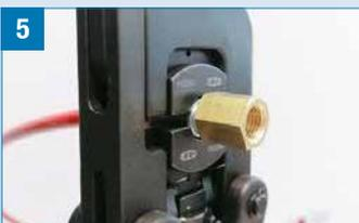
5 Crimp the ferrule with the battery crimping tool. The pliers' die must cover the whole ferrule length.
