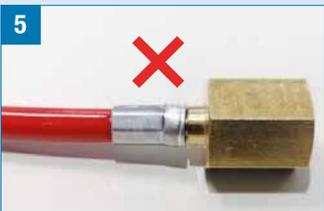
5 Make visual inspections of the fittings after the crimping. The ferrule must be uniformly crimped. In case of an incorrect crimping you have to cut the hose and retry with a new ferrule.
