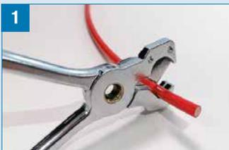
1 Cut the hose at the required length using the proper hose cutter. The cut must be perpendicular to the hose's longitudinal axis.
