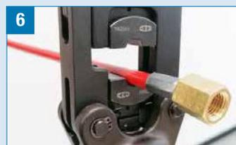
6 Make visual inspections of the fittings after the crimping. The ferrule must be uniformly crimped. In case of an incorrect crimping you have to cut the hose and retry with a new ferrule.
