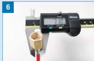
6 Check the crimping diameter by averaging two measurements at 90° and verify that it corresponds with the data shown on the ZEC Crimping Table.
