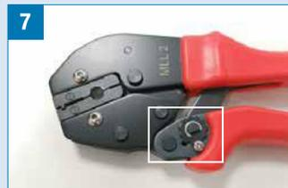
7 If after several uses the measured crimping diameter tends to increase, adjust the gear of the plier.
