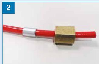
2 Insert the ferrule with the incision on the side of the cut hose. Move the ferrule along the hose. Insert the nut with the thread on the side of the cut.
