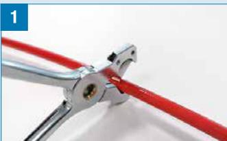
1 Cut the hose at the required length using the proper hose cutter. The cut must be perpendicular to the hose's longitudinal axis.
