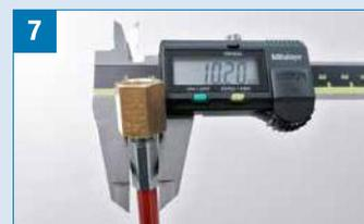
7 Check the crimping diameter by averaging two measurements at 90° and verify that it corresponds with the data shown on the ZEC Crimping Table.
