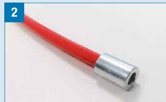
2 Insert the ferrule with the incision on the side of the cut hose.
