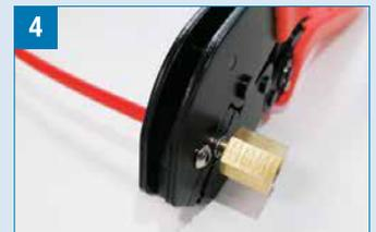
4 Crimp the ferrule with the manual crimping pliers. The pliers' die must cover the whole ferrule length. Keep the pliers completely tight for 10 seconds at least.
